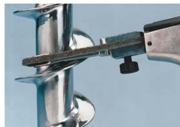
Clean and finish using non-woven nylon belts.
