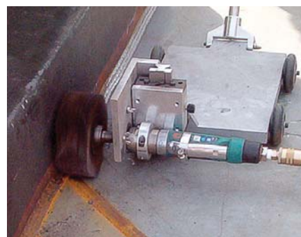
DynaRover cleaning an angle weld.
