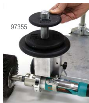
Operator places weights (sold separately) onto optional weight spindle of DynaRover.
