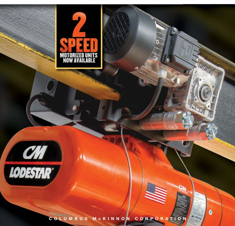
The CM Universal Trolley (UT) is designed to fit virtually all Columbus McKinnon powered chain hoists up to 3 ton capacities, including:
