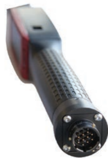
■ Military connector for standard transducer cable
