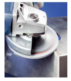
COMBICLICK® unitized discs achieve a very fine, uniform surface finish which, depending on requirements, is a sufficient preparation for high-gloss polishing. Recommended for work on large surfaces on components made of stainless steel (INOX).
