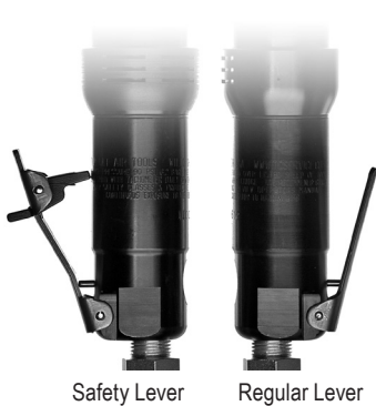
LEVER STYLES FOR 400EH AND 400GEH SERIES TOOLS
