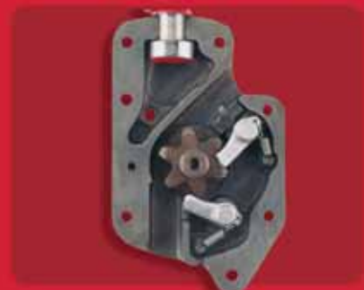
G Series Model (pg.60) Double-Locking Pawl
