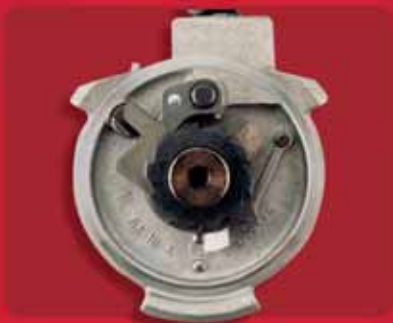
RA Model (pg.59) Ratchet and Pawl Design
