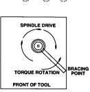
The reaction bar is secured to the tool and braced against the work in the opposite direction of spindle rotation. This will transfer the torque reaction from the tool to the work.
