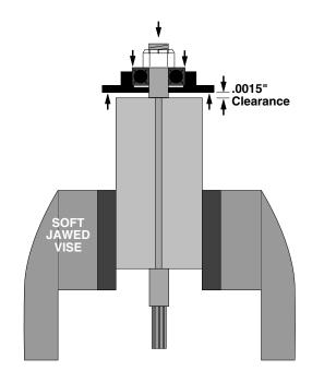
Note: During reassembly of the complete tool, it is important that the motor be free. After the tool is completely assembled, the square drive spindle should turn freely using a small hand wrench. If the spindle does not turn freely, the motor should be checked for proper spacing. Do not run the tool until the spindle turns freely. Failure to do this could result in damage to motor components.
