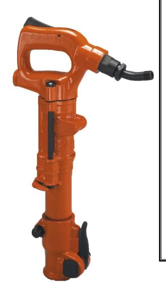
The APT Model 115 Rock Drill works as a drilling tool for drilling holes for anchor bolts and small dowel hole drilling. This versatile tool has a stop rotation feature that converts it from a drilling tool to a percussion tool. It is an ideal tool for light chipping in horizontal and overhead work.
