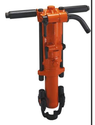
The APT Model 155 Rock Drill is a tough, 60 lb class Rock Drill. This tool can be used in general construction as well as in utility work and plant maintenance. It is designed for drilling through granite, hard faced rock, quarry drilling, and drilling secondary holes for blasting. This tool can also be used with dowel hole drilling machines. Adaptable to wet drilling applications by attaching the APT valve, wet tube and swivel assembly.
